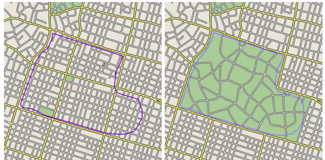
Figure 15: This figure shows that a park can be inserted into an existing street network (left). Notice that the roads in the park region have a sparser density (right).
