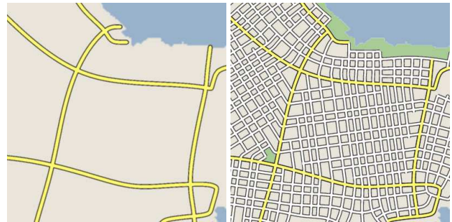
Figure 11: This figure shows a minor road network (right) generated based on the major road network (left)
