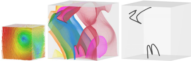
(a) vector field (b) mode surfaces (c) triple degenerate curves Fig. 10: We magnify the center portion of the Bernard cell and show (a) the streamlines of the vector field, (b) the mode surfaces and (c) the triple degenerate curves.
