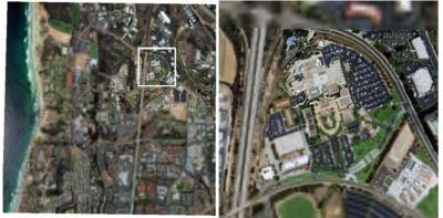
Figure 10: Shows the quad-tree texture at run-time. The camera was positioned very near the surface in the white box. The right image shows the white box region. Note that the texture detail is very high in the center of the white box, where the camera was viewing, but low everywhere else.
