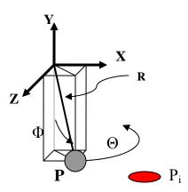
P is the position of the pendulum at the current time. L is the length of the pendulum from the pivot point to the bob. The  $P_i$  are the positions of the magnets and the  $F_i$  are the strengths of the magnets. The total torque on the pendulum is a combination of the magnet forces and gravity acting on the bob as follows:
