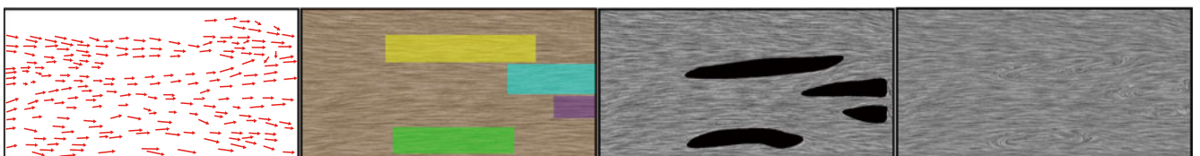
Fig. 8. These are the intermediate flow-field generation results from “Red Cliff” with 1) the initial velocities using extracted strokes, 2) the initial flow field interpolated from the initial velocities, 3) the flow field generated by solving the Navier–Stokes equations, and 4) the complete field after adding whirling fields computed by harmonic functions.
